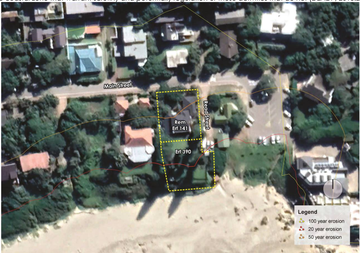
Figure 5: Coastal Management Lines as transposed onto the subject site boundaries (WCG: DEADP, 2018)
