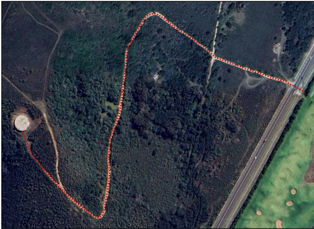
Figure 6: Preferred pipeline route from Goose Valley Reservoir to existing distribution main in N2 road reserve.
