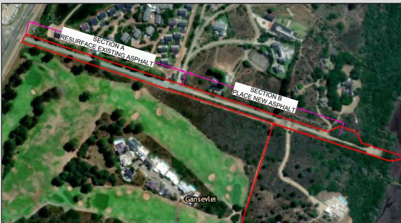
Figure 8: Proposed resurfacing of existing asphalt portions as well as placement of new asphalt on gravel section of Rietvlei Road (Vita Consulting Engineers, 2023).
