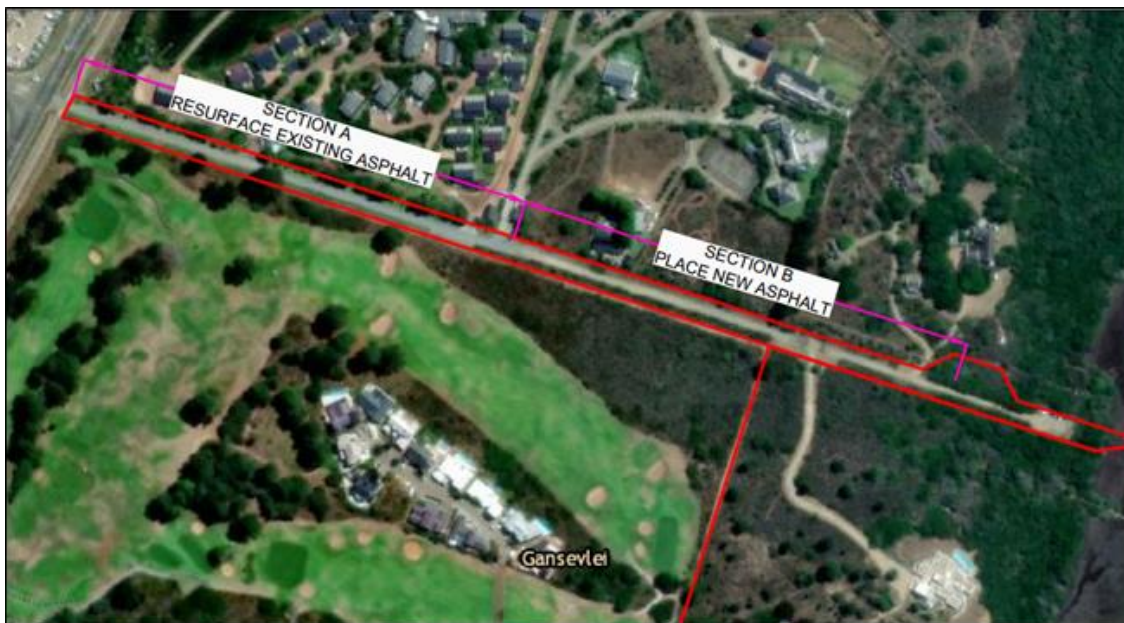
Figure 7: Proposed resurfacing of existing asphalt portions as well as placement of new asphalt on gravel section of Rietvlei Road (Vita Consulting Engineers, 2023).
