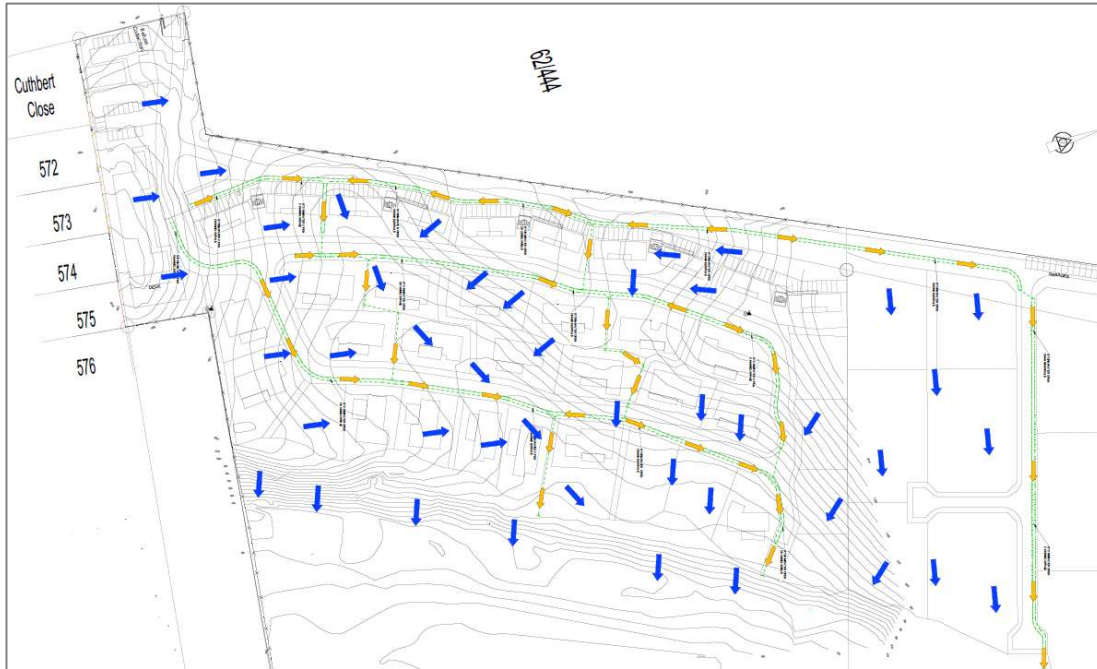
Figure 7-1: Overland drainage patterns
