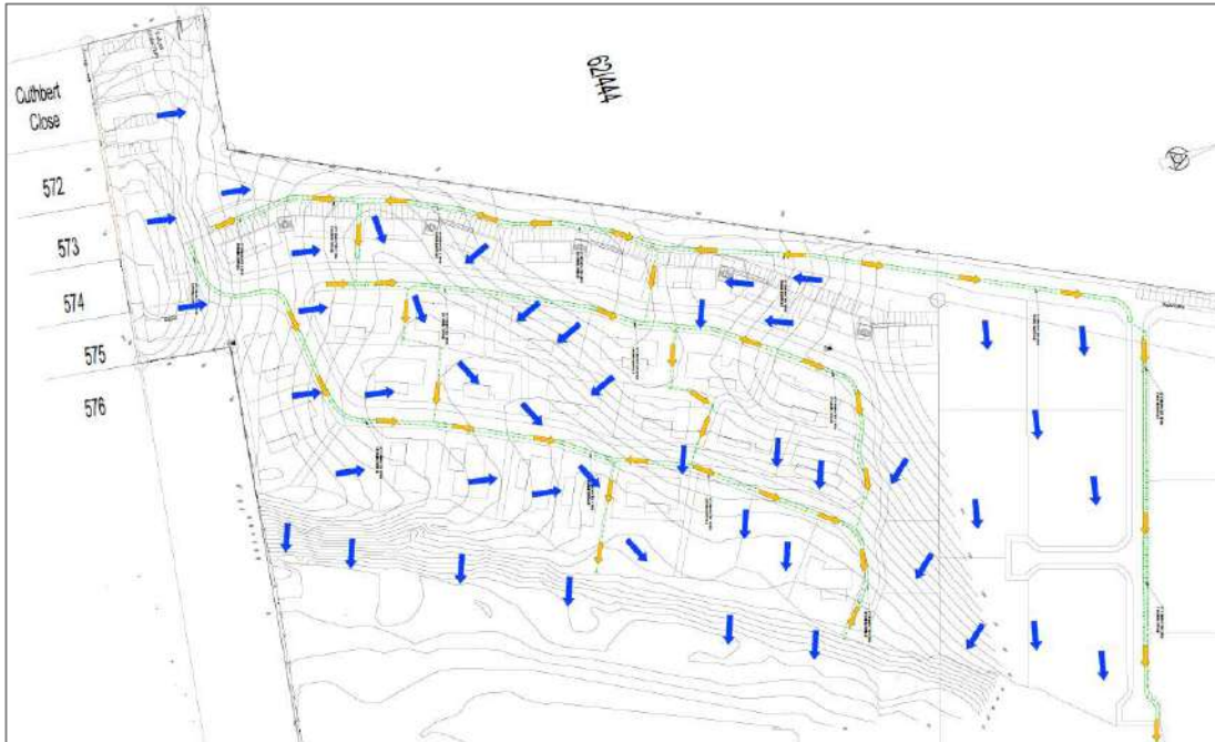
Figure 7-1: Overland drainage patterns
