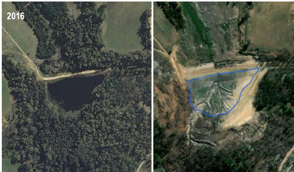
Figure 2. Aerial pictures depicting Bosse Dam in 2016 and post-maintenance in 2019 including an outline of the original dam area.
