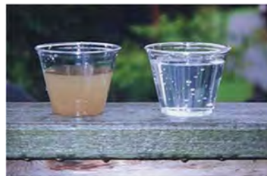
Turbid and Clean Storm Water
