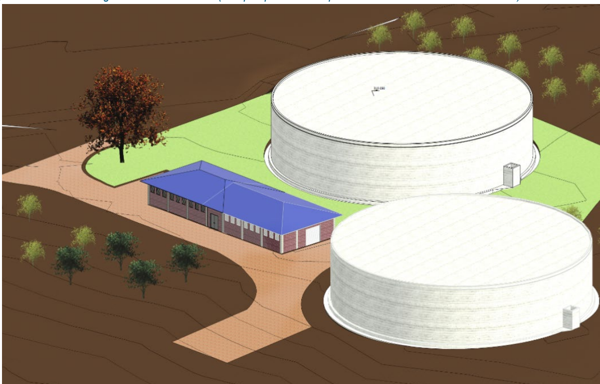
Figure 27: Rendering of reservoir site showing proposed Phase 1A reservoir and pumpstation as well as future phases
