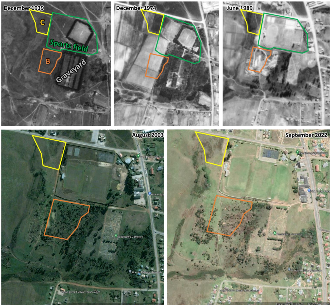
Figure 9: A series of historical imagery sourced from the CD: NGI geospatial portal. The yellow polygon indicates the approximate position of the alternative option C, and the orange polygon indicates the approximate location of the preferred option B area for the proposed development. The green polygon shows the approximate area covered by the sports field in older images.
