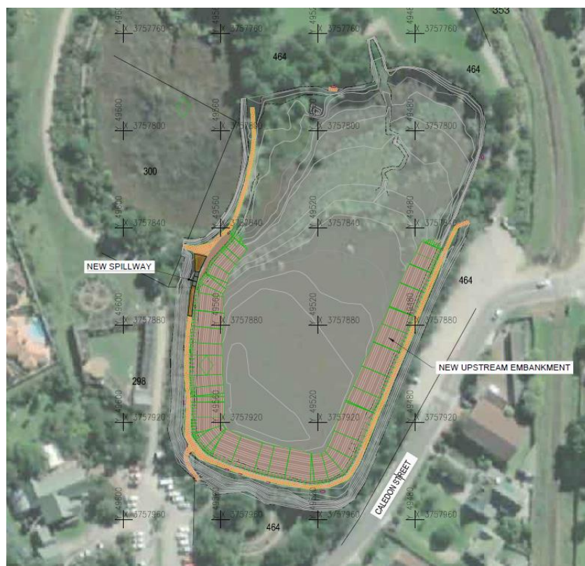
Figure 4. Surveyed layout of the dam relative to surrounding area indicating location of the existing spillway to be upgraded (SMEC, 2023).
