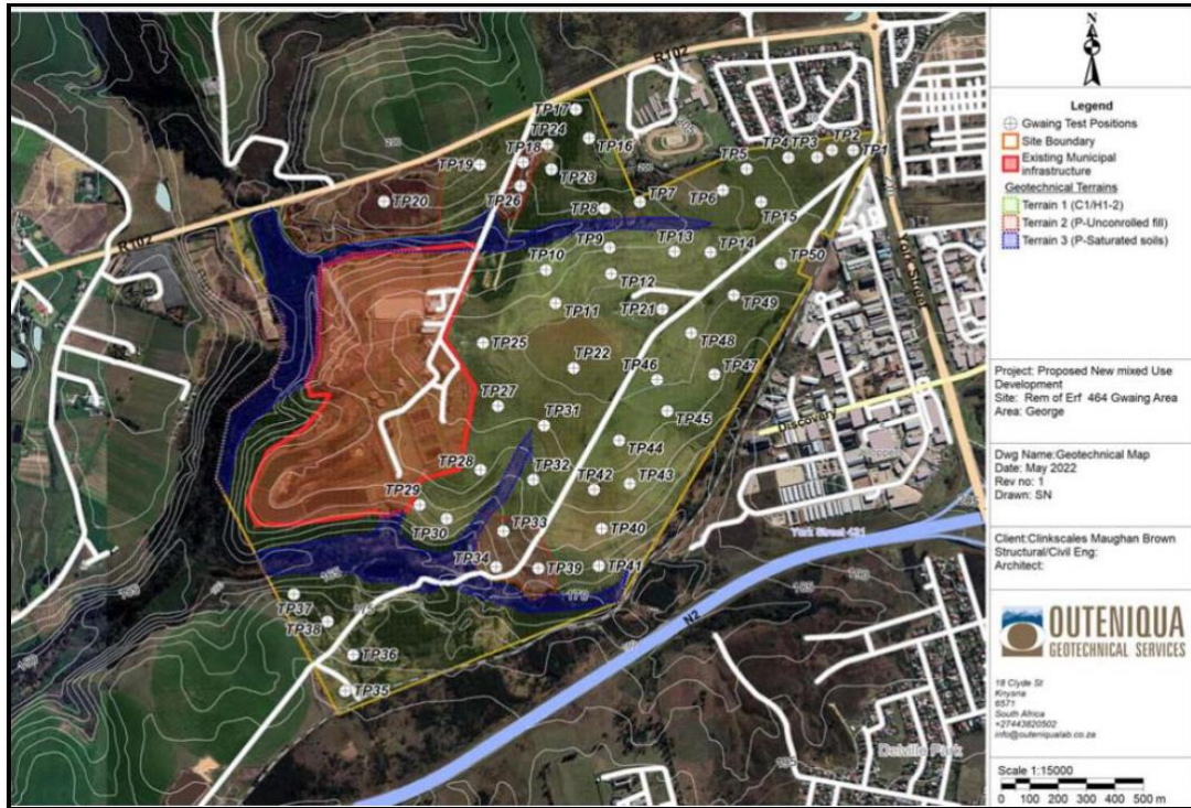
Figure 18: Geotechnical test pit locations across the study area (Source: Outeniqua Lab 2023).
