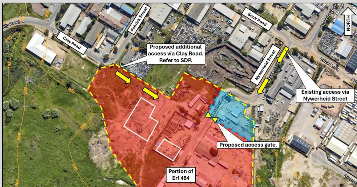
Figure 10: Existing and newly built access roads to the George Municipality Civil Engineering Services Depot (Urban Engineering, 2025).
