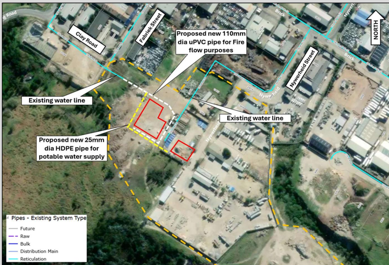
Figure 8: Proposed water supply infrastructure (Urban Engineering, 2025).
