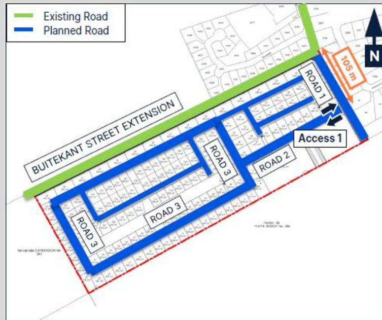
Figure 4: Proposed site access via extension of Buitekant Street as per the Traffic Impact Assessment (Source: SMEC 2022).
