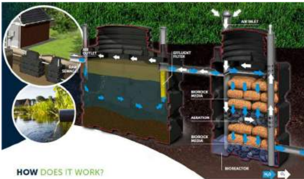
Figure 2 Typical on-site Ecorock bioreactor plant
