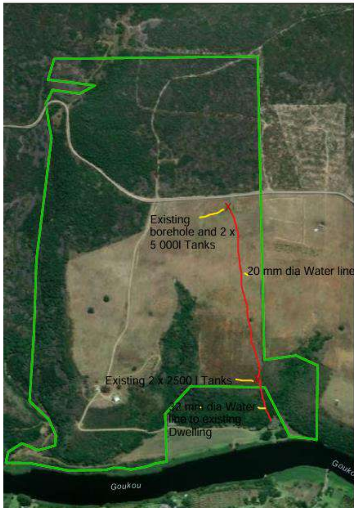
Figure 3: Existing water supply
