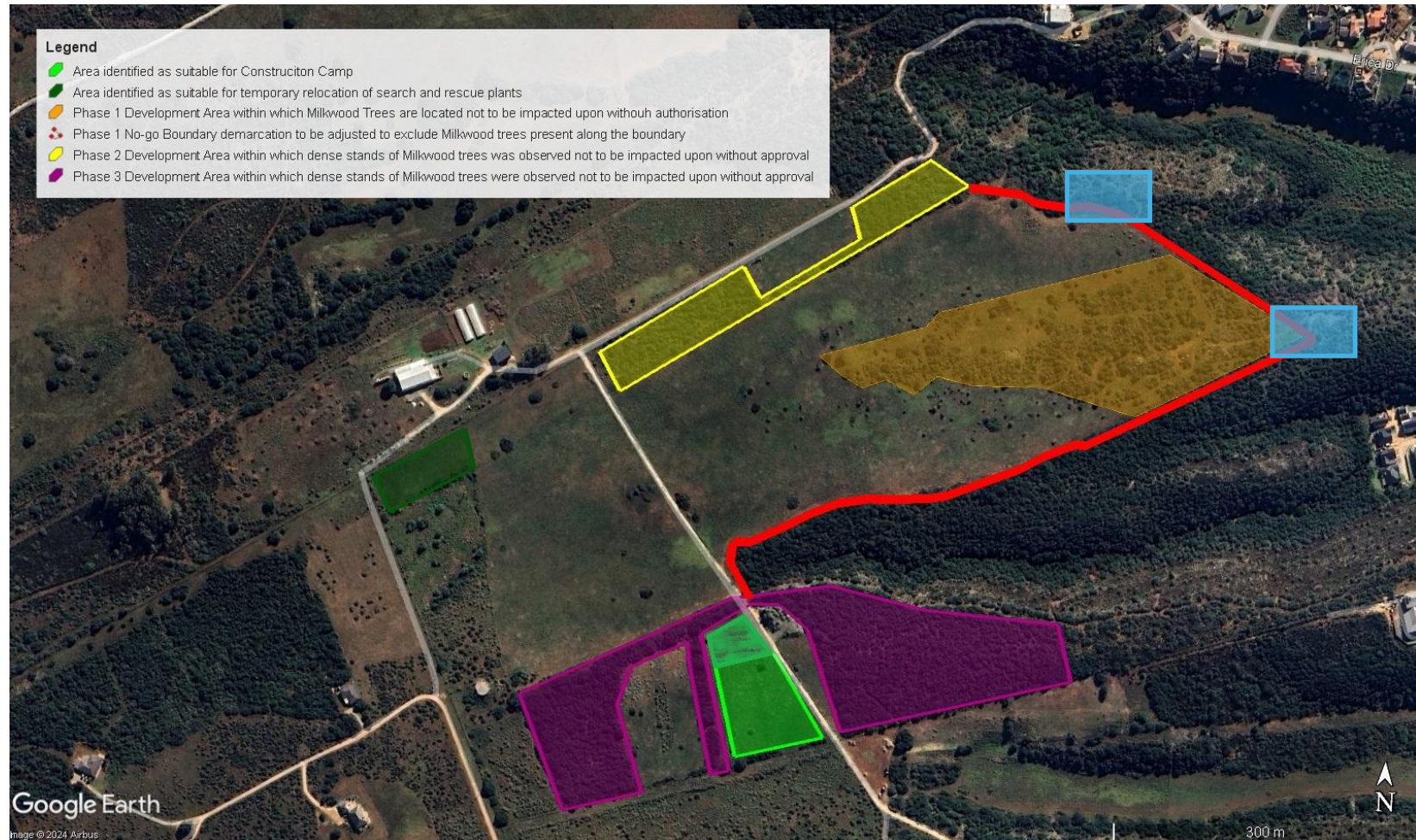
Map 1: July 2024 ECO map for indicating areas where Milkwood trees were observed and to be avoided; proposed construction camp placement; proposed search and rescue plants temporary placement. The blue squares on the map above shows where encroachment into the no-go areas have occurred, as per the recommendations no-go demarcation must remain reinstated as per original demarcation done by the land surveyor and the impacted no-go area must be monitored for rehabilitated
