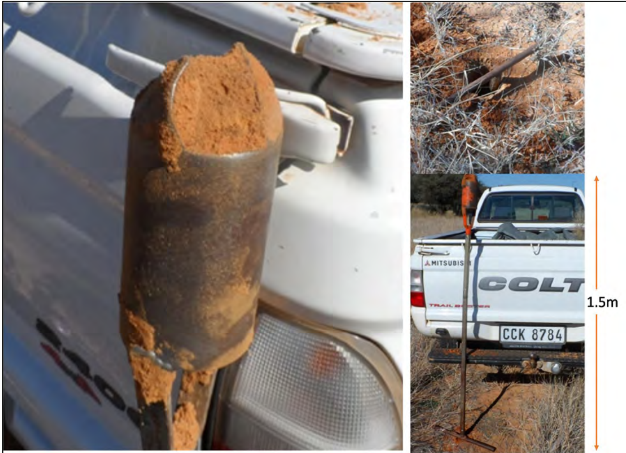
Figure 7: Hand held auger with soil sample
