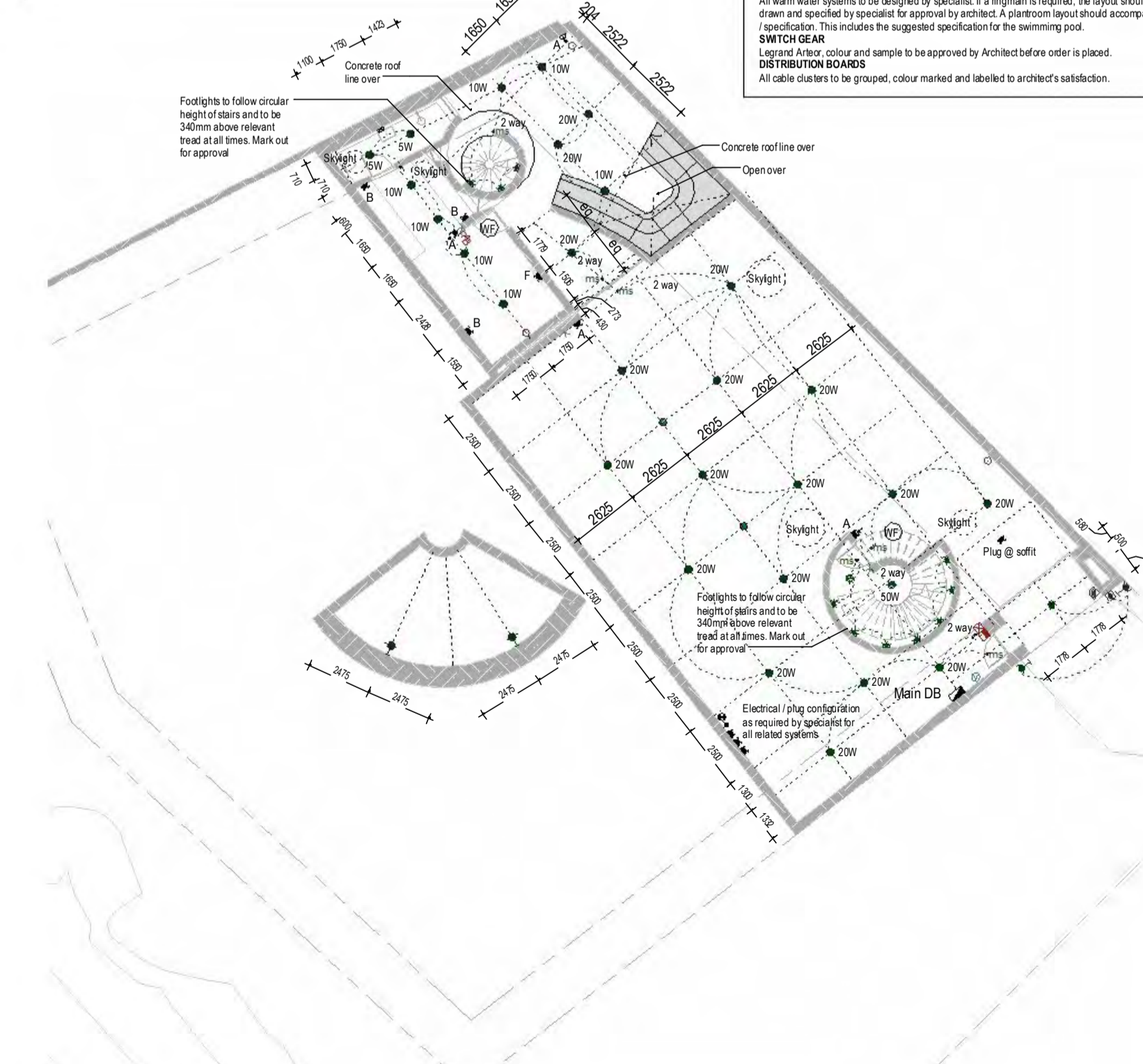
L-1_Basement Floor Plan - Electrical layout SCALE 1:200
