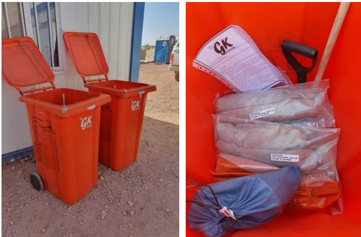
Figure 9: Example of a hydrocarbon Spill Kit to be in place within the site camp.
