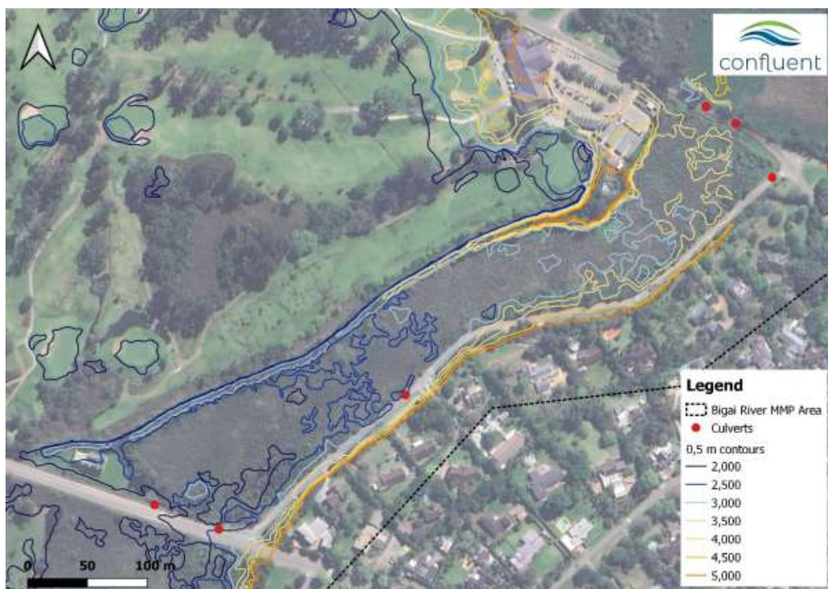
Figure 9. Contours of the Bigai River between Howard Street and Wilson Street in relation to culverts. Based on 2013 Lidar survey of coastal areas (DEA&DP).
