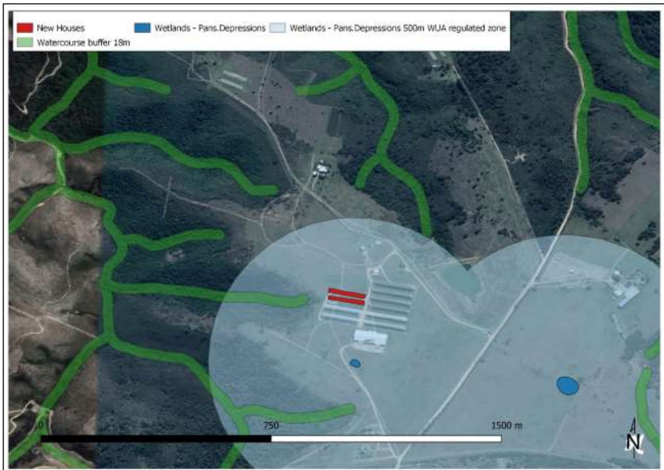
Figure 4: Delineated extent of the pans, known watercourse with 18m buffer and 500m WUA regulated zone in relation to the proposed houses
