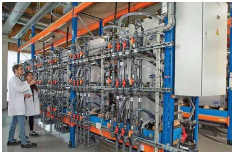
FIGURE 2.3.2.2 – Typical Battery Cell and Stack Set-up
