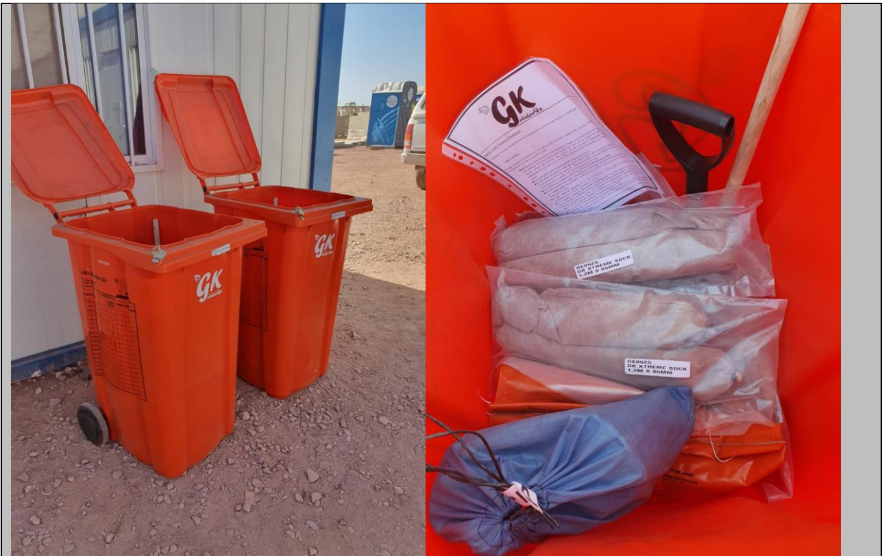
Figure 12: Hydrocarbon Spill Kits must be in place within the site camp and in the field within 500 m of any drilling or ramming activity.
