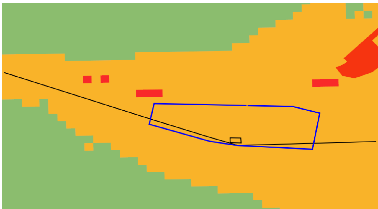
Figure 2. The assessed area (dark blue outline) and grid connection infrastructure (black polygon) overlaid on agricultural sensitivity, as given by the screening tool (green = low; yellow = medium; red = high; dark red = very high). The screening tool's low to medium sensitivity is confirmed by this assessment.
