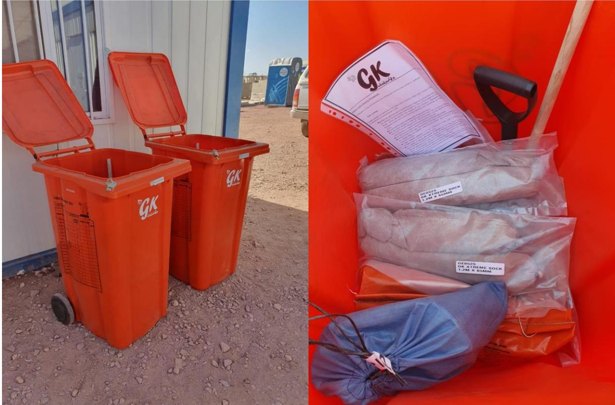
**Figure 14:** Hydrocarbon Spill Kits must be in place within the site camp and within the BESS and Substation construction area.
