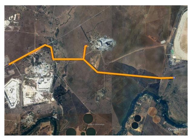
Figure 7: Showing Grid connection infrastructure including powerline (orange polygon) and Eskom Switching Station (blue Polygon) that will be subjected to a separate environmental application to be administered by the provincial authority.
