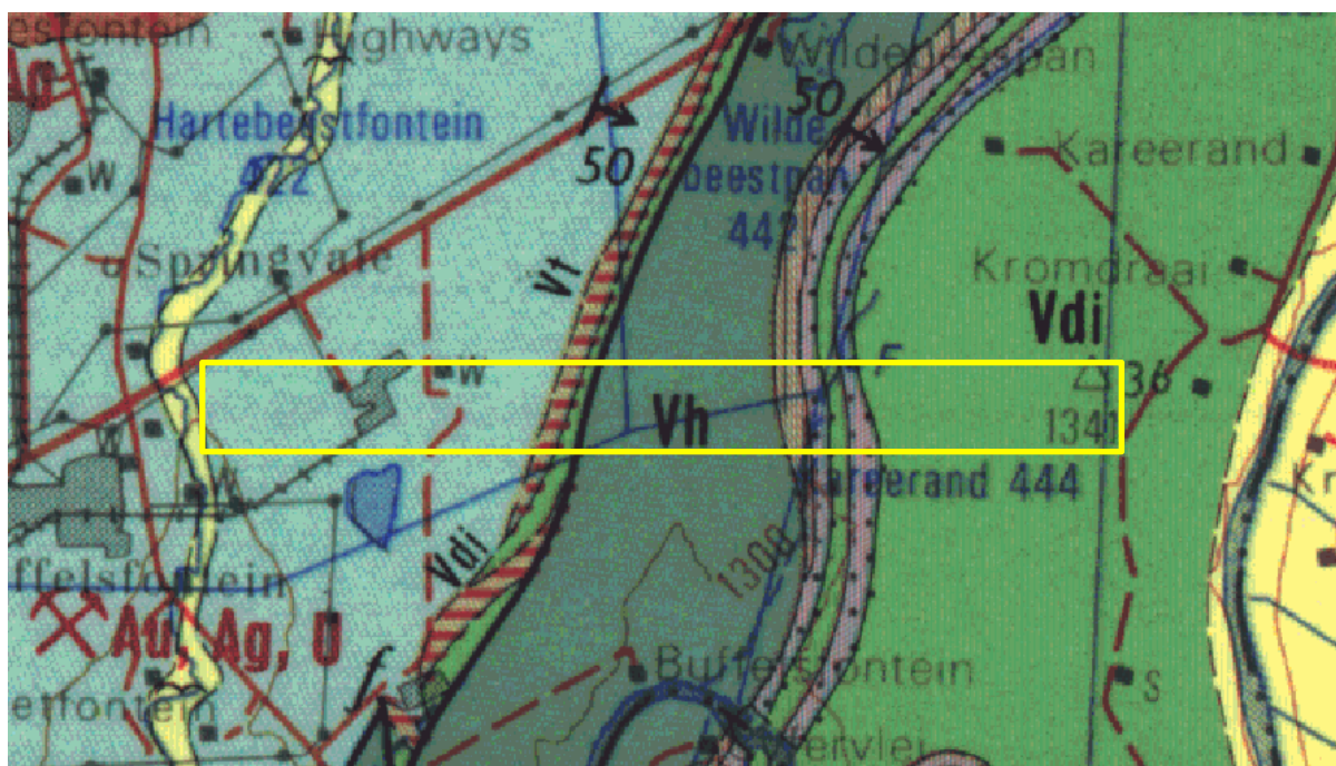
Figure 4: Geological map of the area around the Kareerand BESS site, access road and grid connection within the yellow rectangle. Abbreviations of the rock types are explained in Table 2. Map enlarged from the Geological Survey 1: 250 000 map 2626 West Rand.
