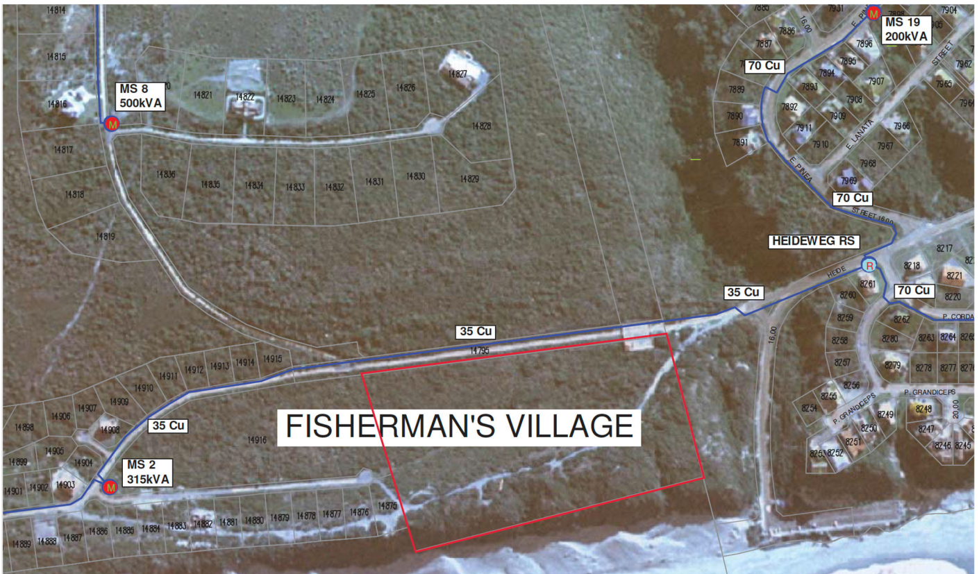
Plan 1: Existing Medium Voltage Network and site location in red
