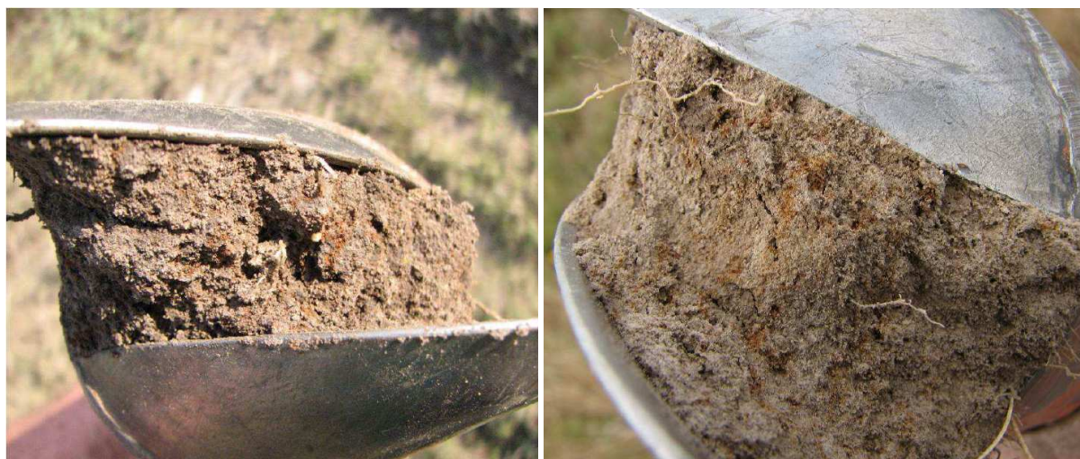
Figure 2: Red and orange mottles observed within soil matrix of delineated wetland area
