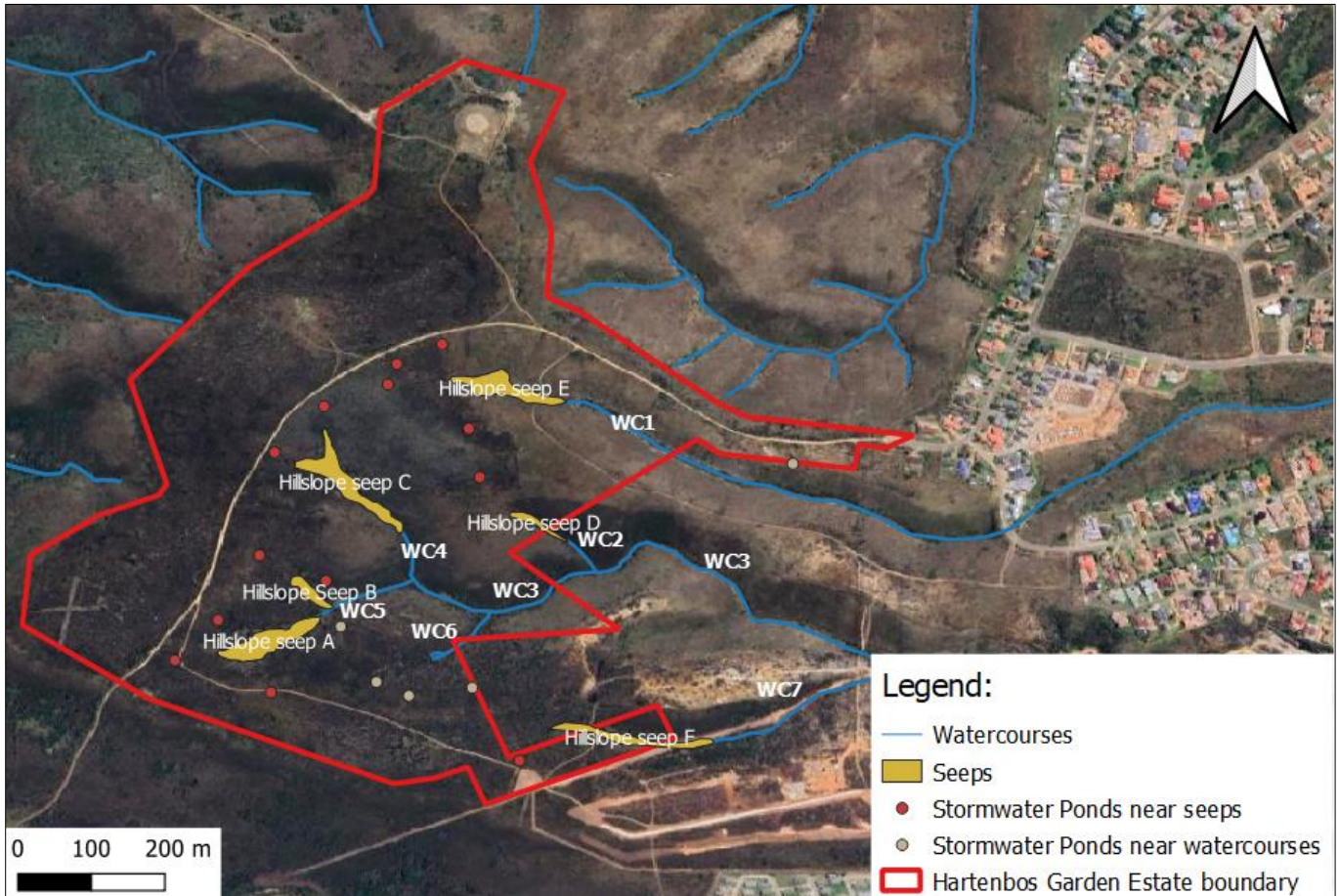
Figure 5: Location of the stormwater retention ponds potentially affecting seeps and watercourse within the study area. These points have been registered as water uses in terms of Section 21 c and i of the NWA.
