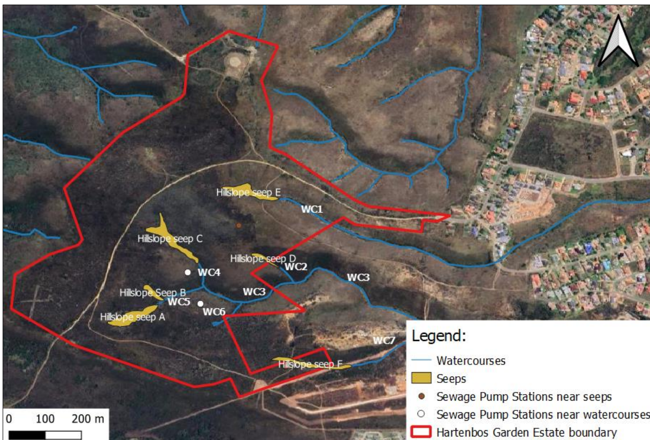
Figure 4: Location of the sewage pump stations potentially affecting seeps and watercourse within the study area. These points have been registered as water uses in terms of Section 21 c and i of the NWA.
