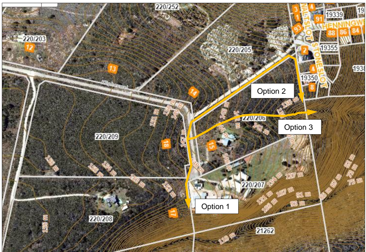
Figure 10: Three external stormwater options on eastern boundary.
