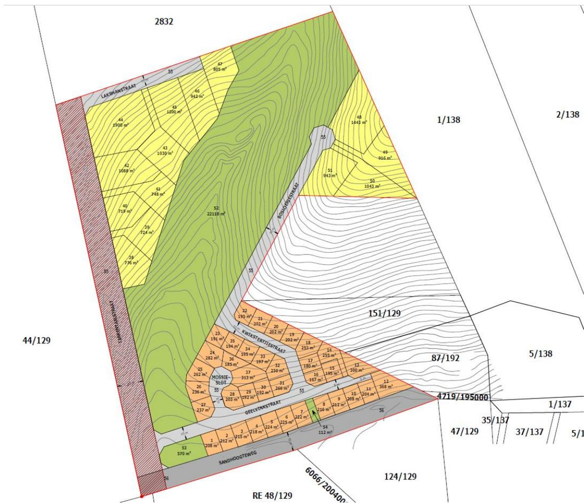
**Fig. 2:** The non-mitigated alternative SDP, with development focussed in three clusters, and the drainage line as a green space bisecting the development.
