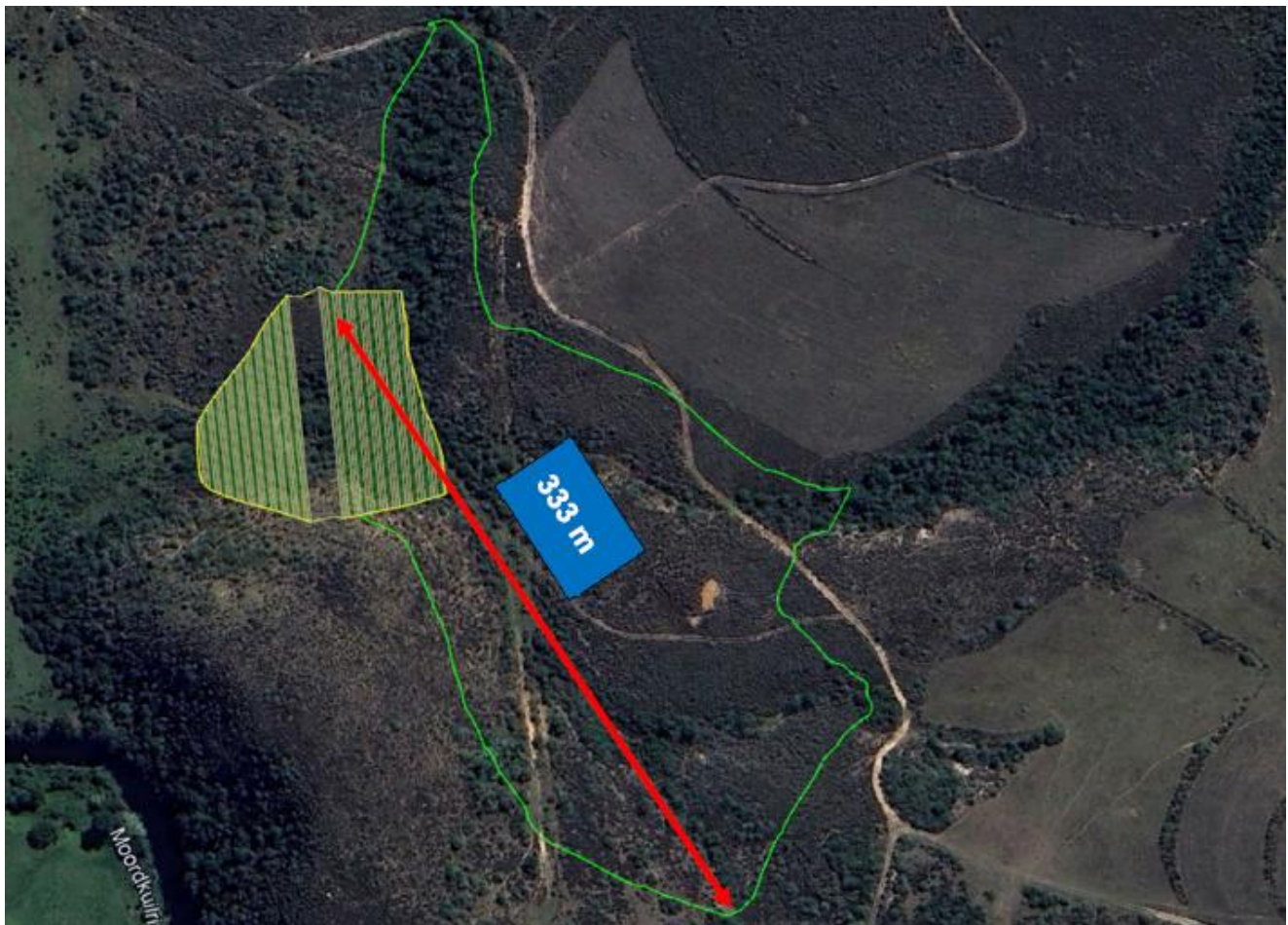
Figure 5: Consideration has been given by the Engineers for the expected fetch in a north-western wind direction which influences wave height and run-off of waves inside of the dam to help inform dam safety design.
