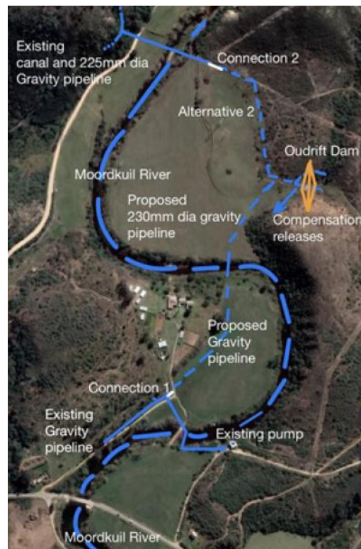
Figure 14: Two different pipes as feeder line and discharge/gravity line.
