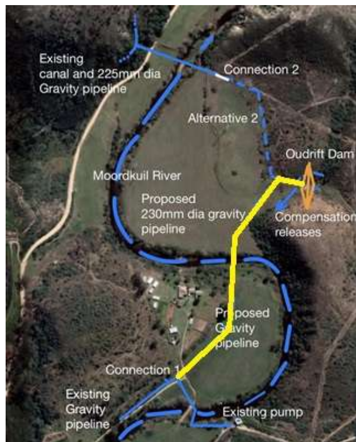
Figure 34: Preferred Water Supply Pipeline Route
