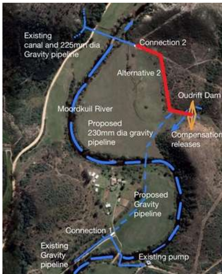
Figure 35: Water Supply Pipeline Route Alternative 1
