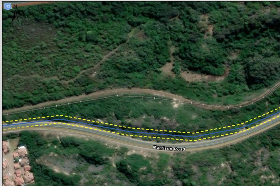
Figure 13: Preferred Standard Trenching Route Alignment.
