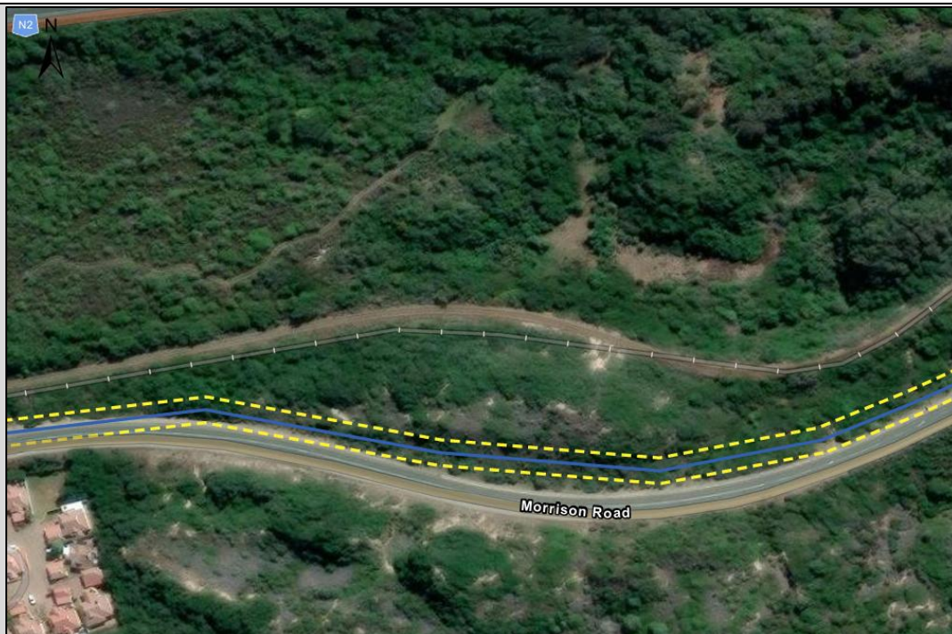
Figure 31: Preferred Standard Trenching Route Alignment.
