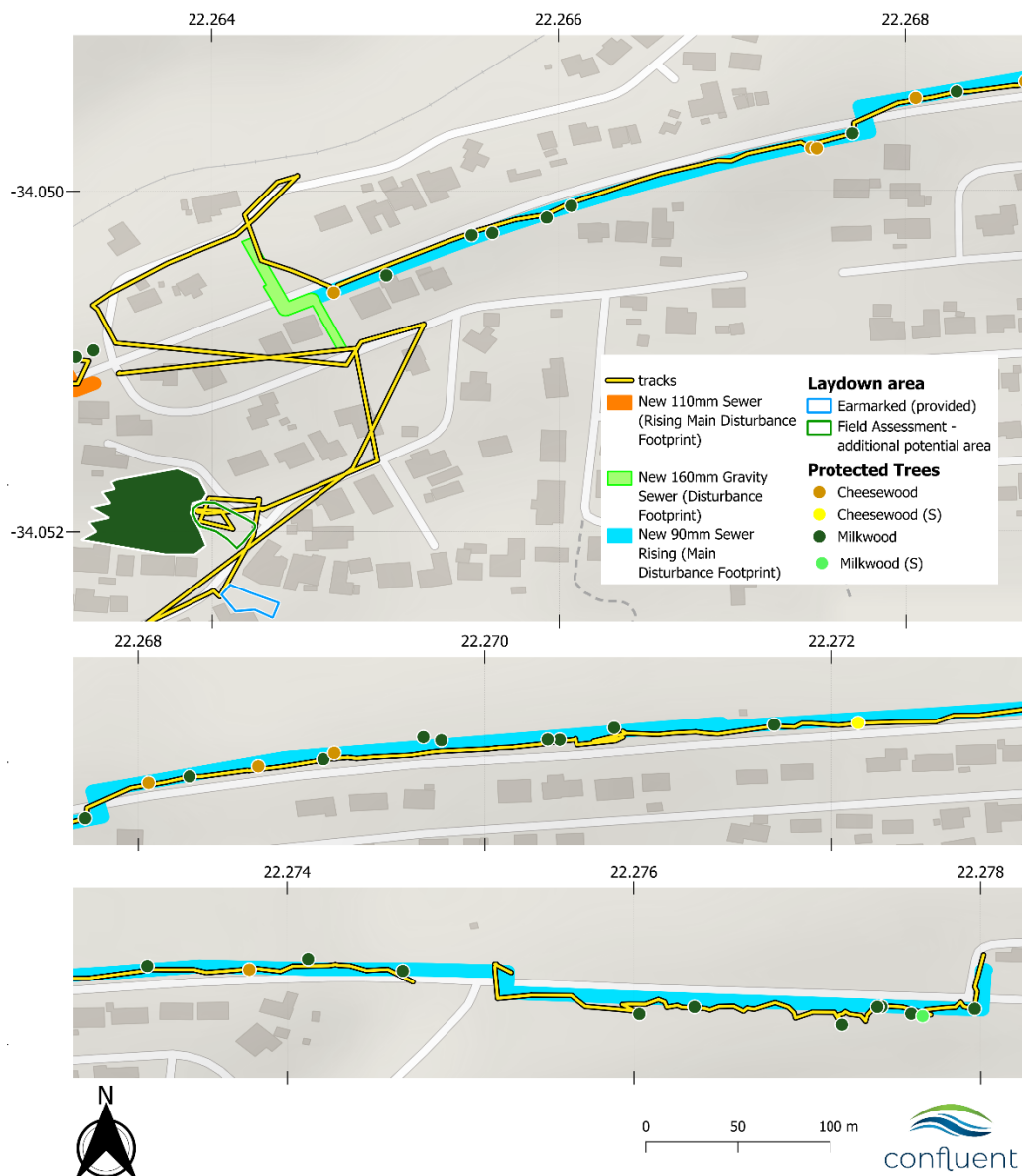
Figure 22: An illustration of the track and protected trees observed during the site assessment for the eastern half of the sewer line proposed. (S) indicates a seedling.
