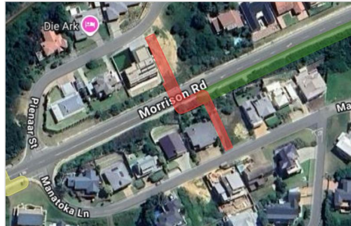
Figure 6. Alignment of the Ø160 mm gravity line from the new manhole in Pienaar Street to the existing manhole in Manatoka Lane ( \pm 0.1 km). The 7 m disturbance envelope is shown.
