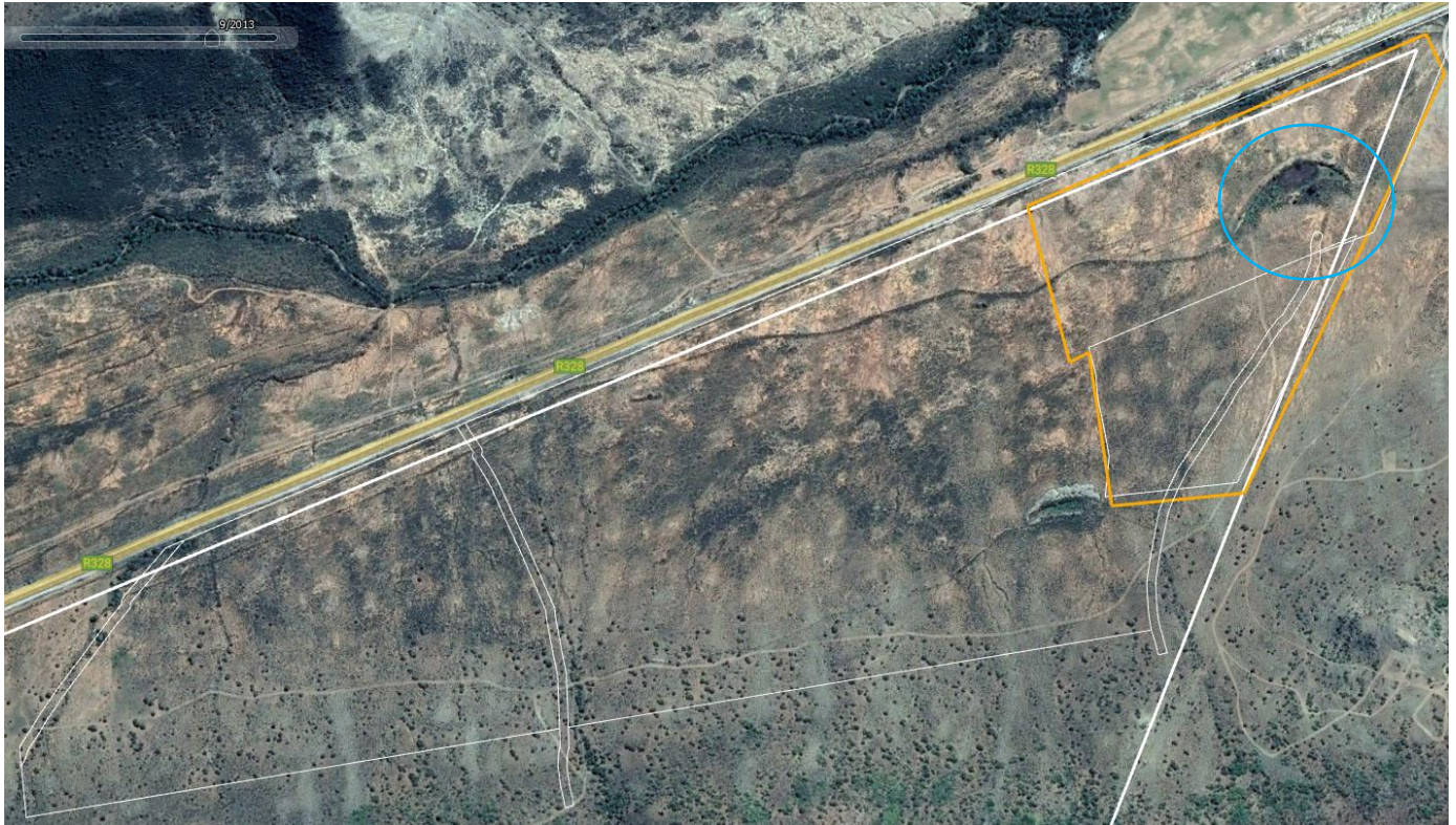
Figure 6: Google aerial image (2013) showing the small off-stream dam fed by a cut-off canal (dark line along the northern portion of the site) and unnamed tributary feeding into the off-stream dam subsequently transformed for cultivation (Source: Google Earth).
