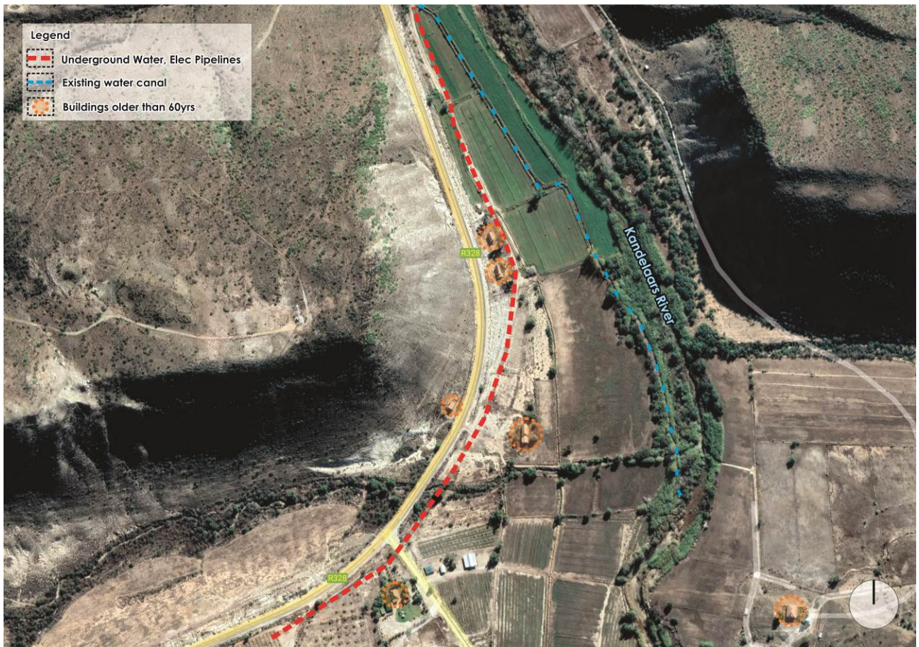
Figure 5: Approximate alignment of underwater pipeline in relation to existing water canal and historic structures located along the Kandelaars River valley, directly northeast of the subject farm (GoogleEarth, 2020, as edited)
