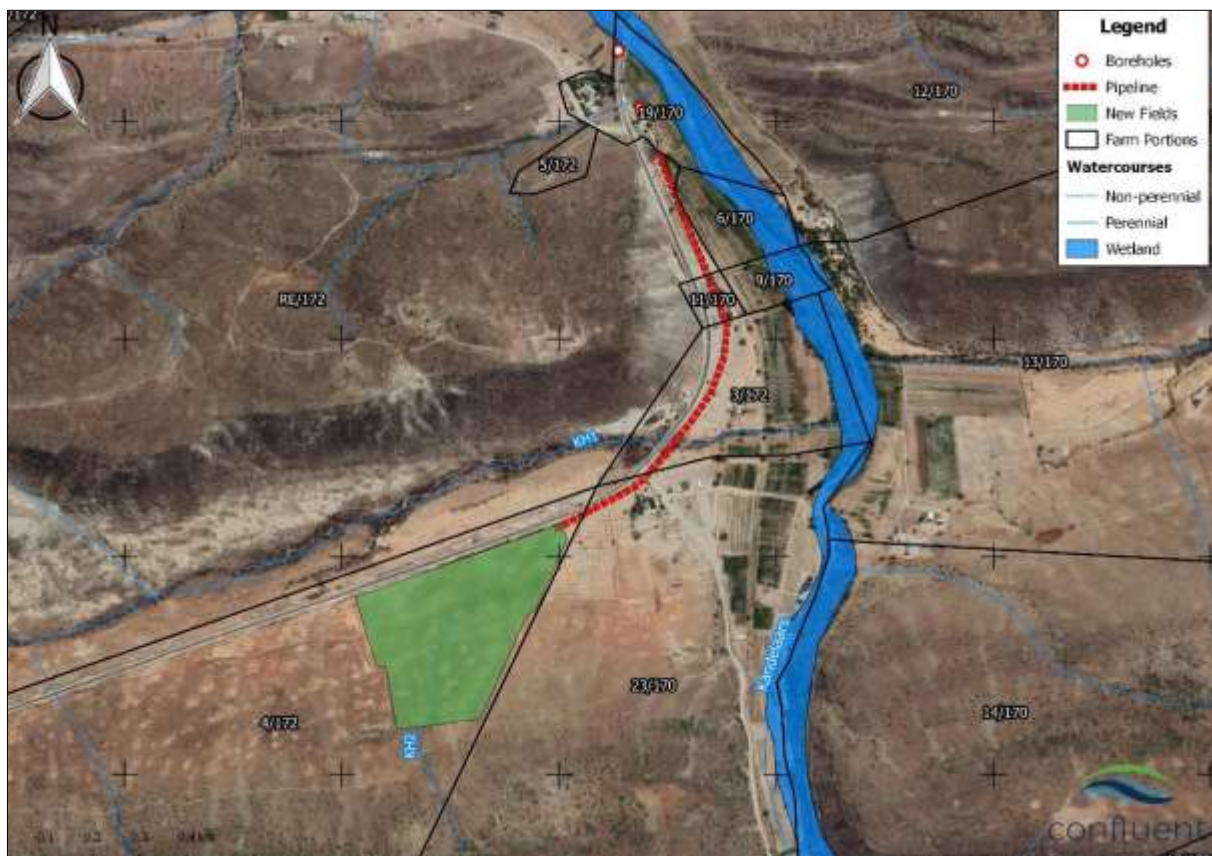
Figure 2: Aquatic map showing the affected watercourses on site (boreholes KH1 and KH2) and 5m buffers of those watercourses (extracted from Aquatic Assessment Report, 2022).
