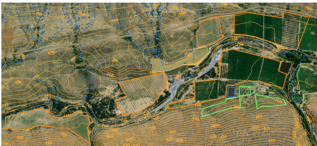
Figure 10. 5m site contours and mapped watercourses overlaid with feedlot areas and existing fields (from Cape Farm Mapper).
