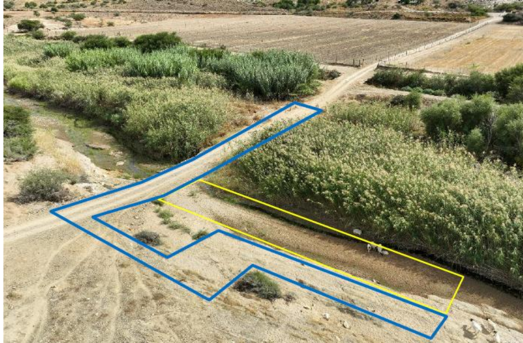
Figure 17: Extent of vehicle movement (BLUE) and upstream excavation (YELLOW) during reconstruction.
